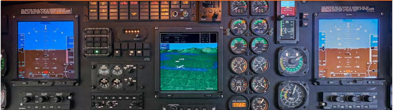
The flight information display and flight management system upgrade replaces analogue systems with three 8.9" digital 'smart' displays, increasing operational capability, reducing issues with aging instruments, and eliminating the costs of replacing or maintaining older analogue displays. This upgrade is a cost-friendly option for operators who desire the modern S-76D-like avionics look and feel for other S-76 variants including the S-76A, C, C+, or C++ models.
