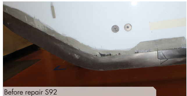
Replacement of SS-strip on leading edge MK-2
