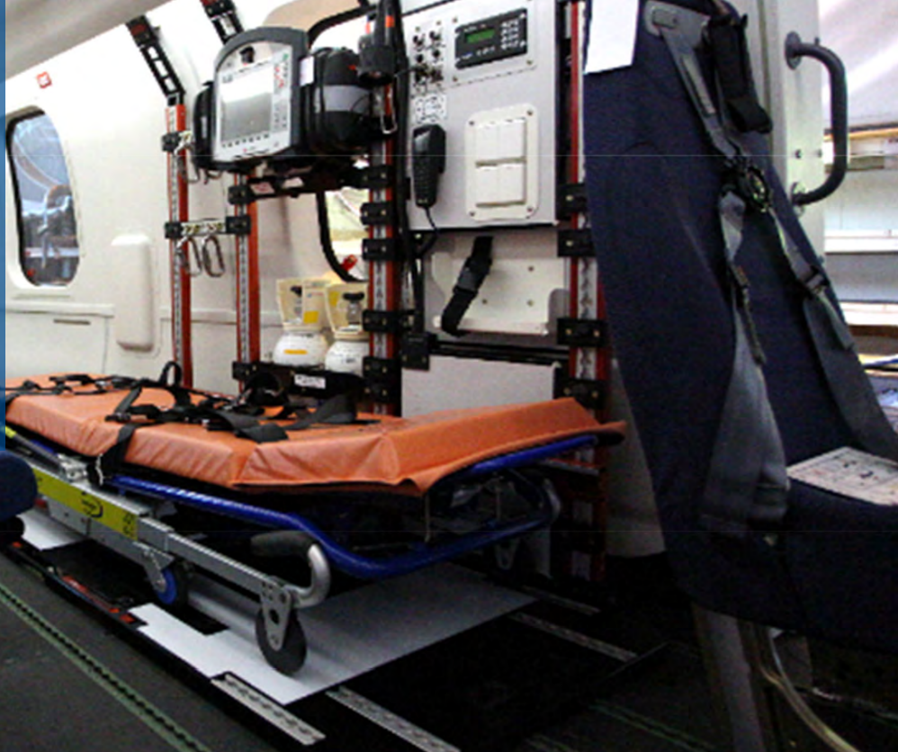
SAR CABIN CONFIGURATION INCLUDING EQUIPMENT WALL
