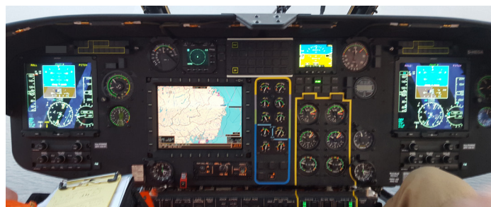
FLIGHT INFORMATION SYSTEM UPGRADE INSTALLED IN AS332
