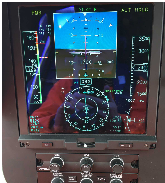
UNIVERSAL EFI-890H DISPLAY WITH KEY FLIGHT INFORMATION
